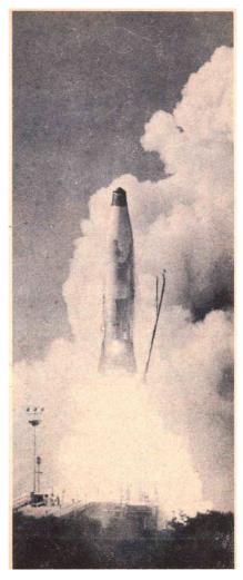
Fig. 5: (Left) Jupiter-C, carrying Explorer satellite in its note, talcing off
